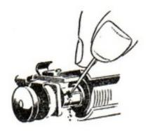
KEEP COMMUTATOR SEG-MENTS CLEAN WITH SMALL HOUSEHOLD PIN. BRUSH WITH METHY-LATED SPIRIT TO REMOVE CARBON DIRT
