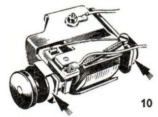
OCCASIONALLY APPLY A VERY SMALL AMOUNT OF OIL TO PADS ON MOTOR
