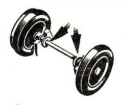
APPLY LIGHT GREASE TO REAR AXLE BEARINGS AT PLACES INDICATED
